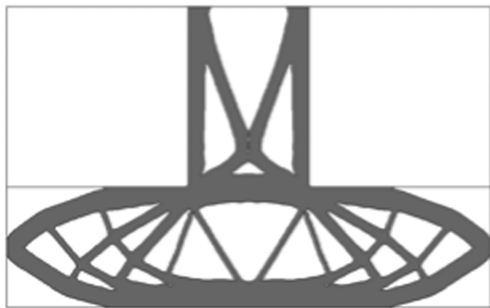
Fig. 6 Double hook example: a) design domain and initial topology, b) deterministic solution, and c) robust solution.
